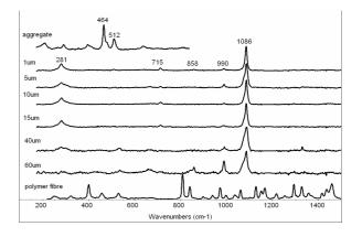
Fig. 3 Raman spectra of quartz/feldspar aggregate, cement matrix of various distances from quartz/feldspar aggregate surface and spectrum of PP/PE polymer
