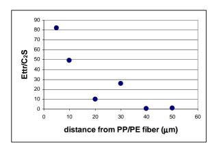
**Fig. 7** Relative concentration of ettringite as a function of the distance from PP/PE fibre surface
