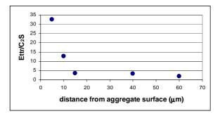
Fig. 4 Relative concentration of ettringite as a function of the distance from quartz/feldspar aggregate surface
