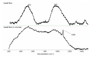
Fig. 10 Raman spectra of parent basalt fibre and the fibre deposited in cement matrix
