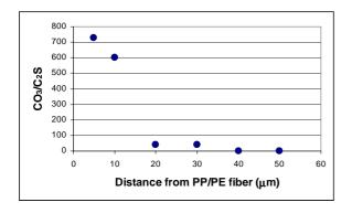
Fig. 8 Relative concentration of carbonate as a function of the distance from PP/PE fibre surface
